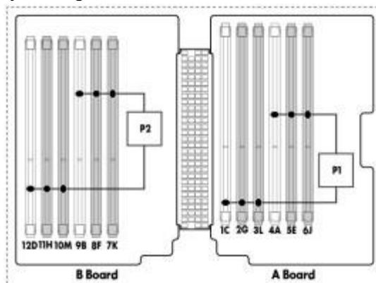
The memory subsystem in this server is divided into channels. Each processor supports eight channels, and each channel supports
